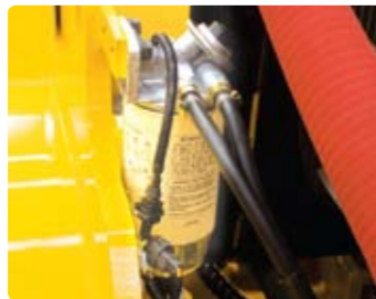
Mechanic friendly fuel filter replacement Highly accessible engine compartment allows for quick replacement of filters.
