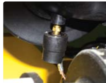
Electrically monitored air filter Air cleaner sensor alerts the operator of a clogged air filter and allows replacement before damage.
