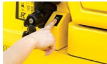
Cabin tilting automatic system Cabin tilting automatic system makes servicing of all power train components quick and easy. An electrically assisted hydraulic actuated cylinder tilts operator cabin to left side about 54 degrees for easy access to inside of truck components.
